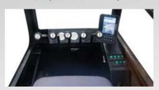
Full vision extra large glass and skylight Indoor space extended for more comfortable working environment Standard 6" color screen with LMI, load data in real-time display Integrated electrical system and throttle control, eco mode
