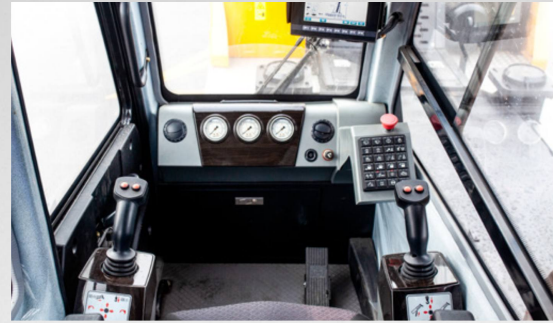
Standard 7" HD screen with LMI, load data in real-time display. All new membrane touch button panel tilted by 45°, status displayed, easy to operate. One button switch of eco and strong modes.
