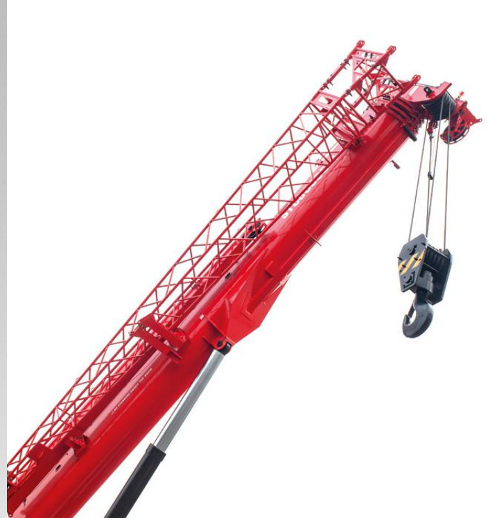
Five section boom welded by high-tensile steel plate, featuring good rigidity. Max. lifting height is lifted to 65m after mounting 17.5m fixed jib. Max. lifting moment 2881kN · m, capacity upgraded significantly.
