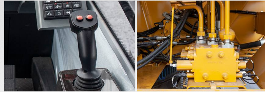
Control precision and stability are enhanced via new generation electrically controlled hydraulic system of electrical joystick and electro proportional main valve.
